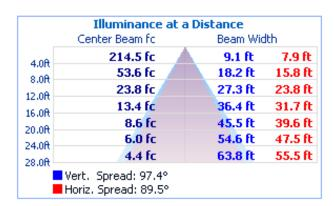
SL80-UM-PFB(DW), 8,000 delivered lumens, tested by Dongbu Lightec Lab, tested in accordance to IESNA LM-79
