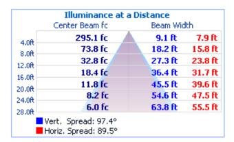
SL110N-UM-PFB(DW), 11,000 delivered lumens, tested by Dongbu Lightec Lab, tested in accordance to IESNA LM-79
